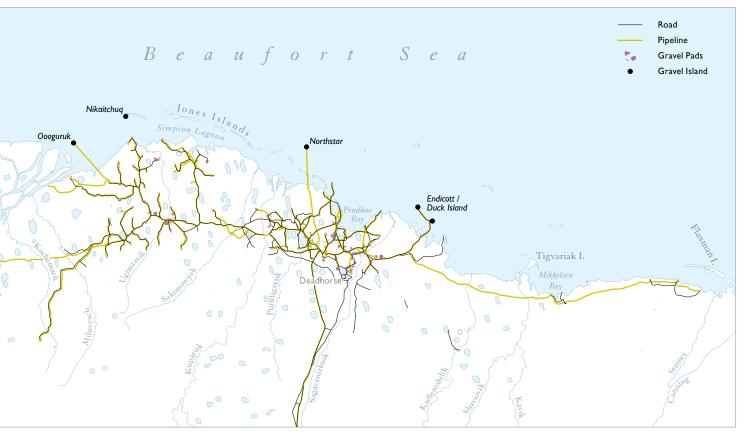
FIGURE 7.3-2. Oil and gas infrastructure (roads, pipelines, gravel pads, and gravel islands) on the North Slope of Alaska.
