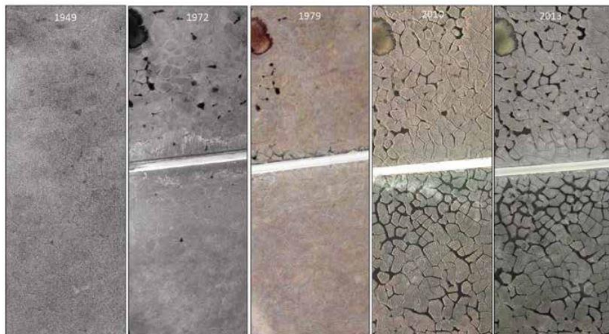
Figure 6. Adapted from Walker et al. (2014). Development of extensive thermokarst after construction of a gravel road. Aerial imagery near Lake Colleen, 1.9 mi (3 km) north of Deadhorse, Alaska.
